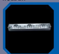
The holder is CNC machined from 4340 steel. A diamond carbide powder is weld-fused to the contact surface ensuring the longevity of the holder in even the most aggressive applications. An end plate is welded to each end of the holder to block contaminants from entering the system.
