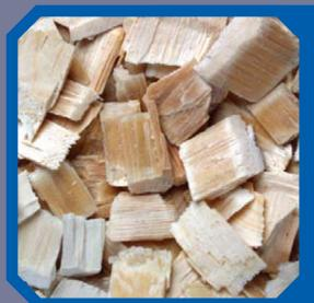
The KPS's innovative Uni-Ridge Knife consistently formulates a uniform chip and provides a smooth transition from the knife across the counterknife. The smooth transition greatly reduces the break up of quality chips into pins and fines. To improve chip modulation the KPS gives you the flexibility to adjust knife attack by simply changing the knives. Now more than ever you have greater influence over your mills chip quality and distribution.
